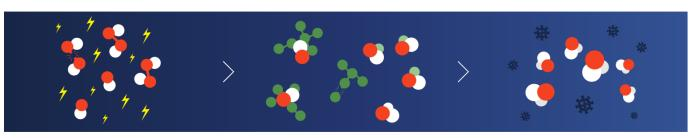
1. UV rays transform hydrogen peroxide into highly reactive hydroxyl radicals.
